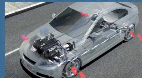
The generator transforms kinetic energy into electrical energy, which is stored in a high-voltage battery.
